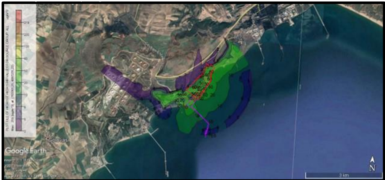
Figure 9-8. Yearly average maximum APCV dispersion of VOC for Scenario-1 (i.e., tanks in the Ceyhan The Project and Associated Facility under controlled operating conditions) during operation
